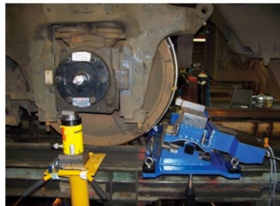
A portable wheel lathe from Delta Manufacturing being used to maintain a railcar wheel.
